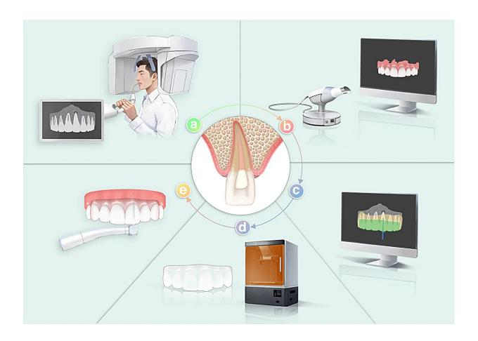
Schematic diagram of SGE a. CBCT scanning b. Oral scanning c. Virtual guide design d. Template printing e. Intra-oral guided drilling. Credit: *International Journal of Oral Science* (2023). DOI: 10.1038/s41368-023-00261-0
